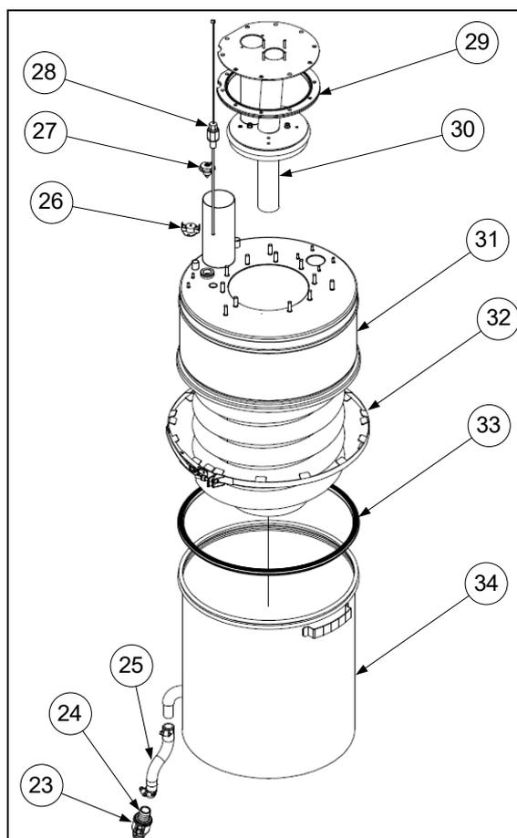
Illustration 53 - Evaporation Chamber Assembly Exploded View
